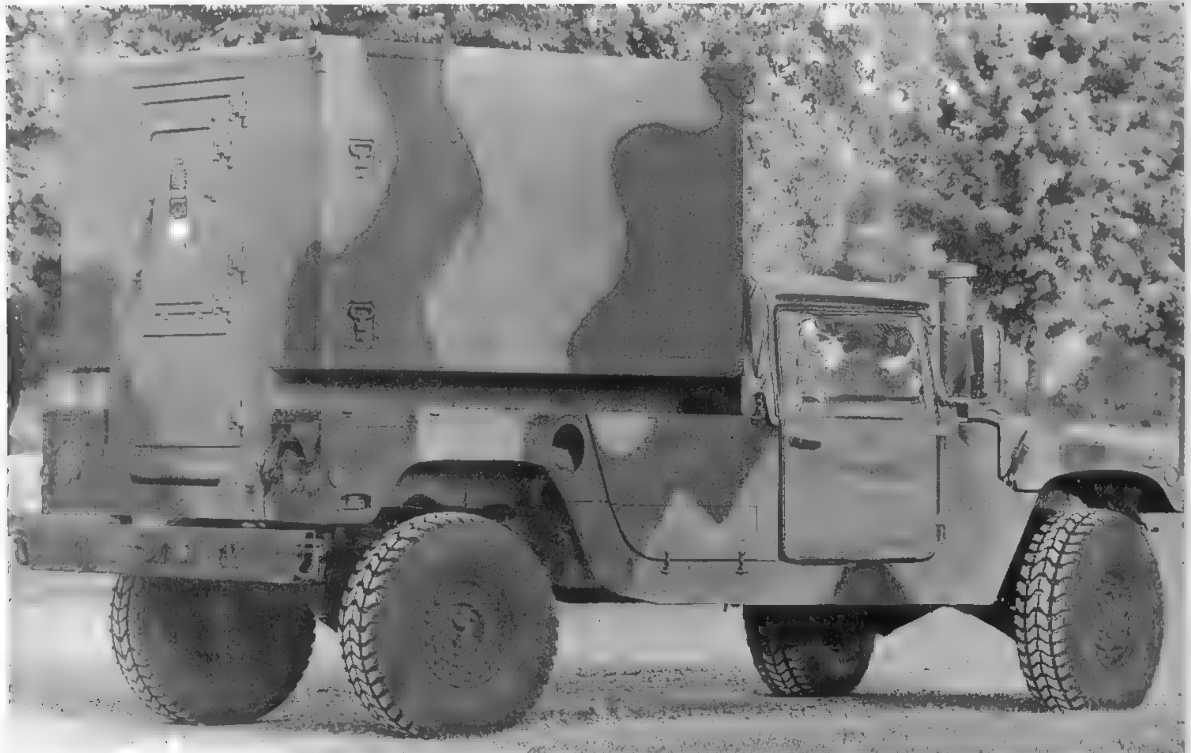
The M1037 shelter carrier was designed to transport the S250 communications shelter. These shelters can be used for communications, electronics, or command purposes and are secured firmly to the vehicle. (Photo courtesy of AM General Corp.)
